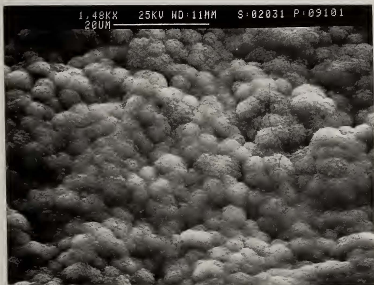
Fig. 3b. Continuous diamond film growth on a surface-treated quartz substrate using gas phase seeding.
