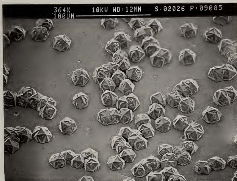
Fig. 3a. Diamond grown on an untreated quartz substrate showing a low nucleation density. Well-defined facets are clearly visible indicating the good quality of the crystals.
