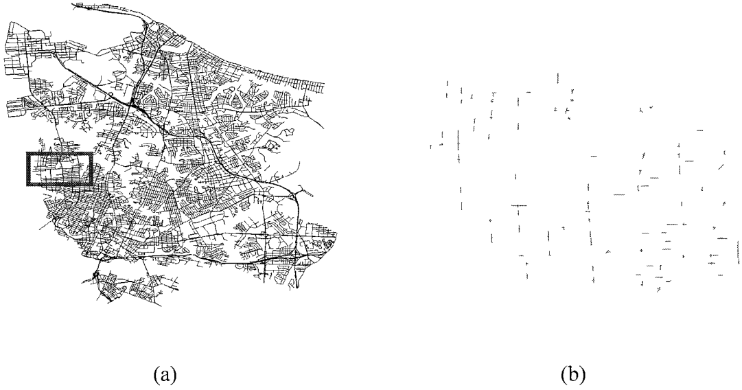
Fig. 3. An example of raw road GIS data. (a) Road GIS data containing all Norfolk street information displayed in ArcGIS. (b) An enlarged view of streets around Old Dominion University is denoted by the red rectangle in (a).
