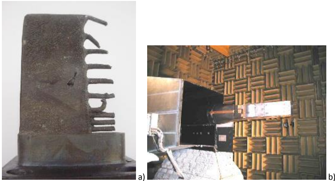
Figure 8 a) The Effect of Flame Impingement on a Temperature Rake, b) High Speed Research Model where the Rake was used. (12)
