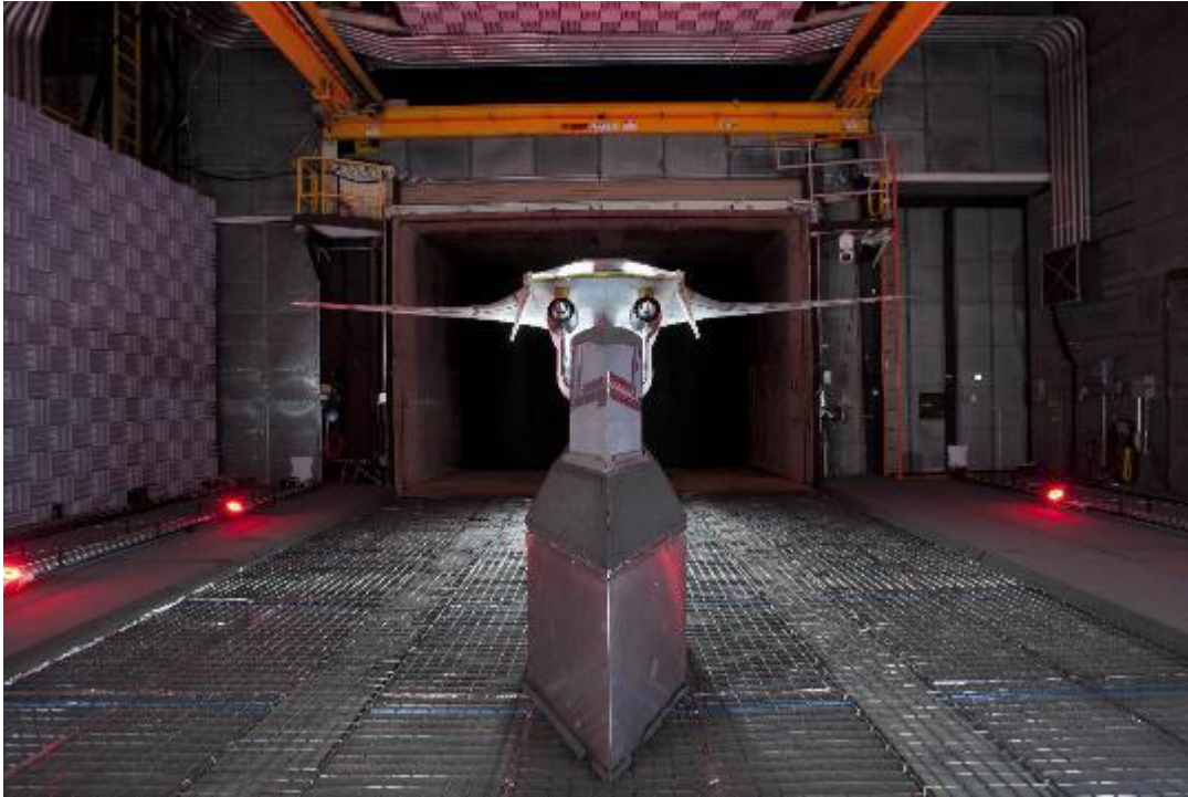
Figure A-4 Aft View of the Hybrid Wing Body Showing the CJES Units. (39)
