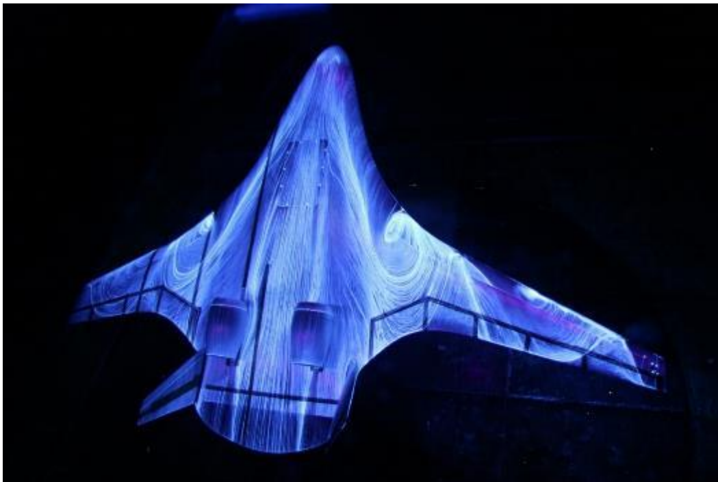
Figure A-6 Oil Flow Visualization of Surface Flow Patterns. (40)
