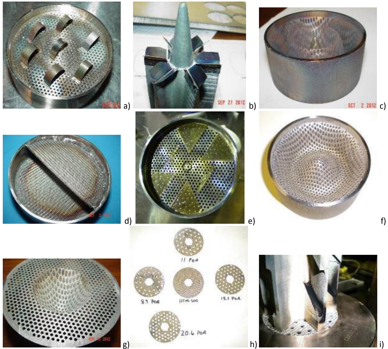
Figure 41 Selected Combustor Change Variations intended to eliminate the Combustor Instability; a) Spot Welded Straps, b) Trailing Edge Fins on the Plug-Vane, c) Double Sinusoid Upstream Face on the Honeycomb Flow Conditioner, d) Staggered Screens to Replace the Honeycomb, e) Baseline Honeycomb with Flow Blocking Wedges, f) Single Sinusoid Flow Conditioner, g) Flat Faced Honeycomb with an Elliptical Dimple, h) Sintered Screen with Hole Patterns for Different Percent Open Areas, i) Location of the Sintered Screen Ahead of the Combustor. (12)
