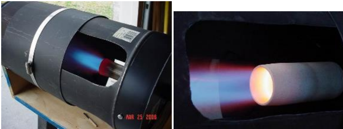
Figure B-2 a) Commercial Off The Shelf (COTS) Torch, b) Torch in a NAVSEA Project Mock-up, c) Ceramic Flame Holder. (12)
