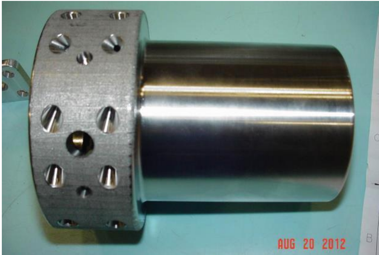
Figure 26 Finished CoCr Combustor Liner. (12)
