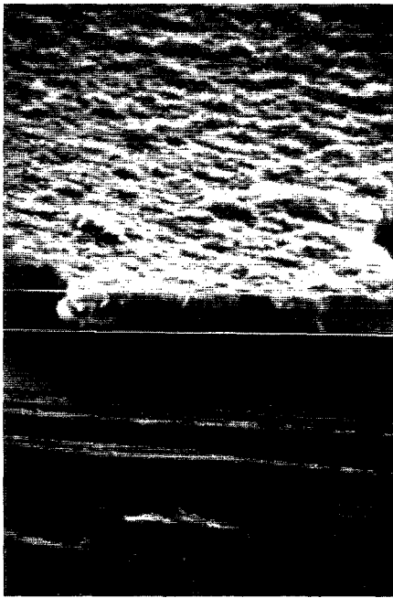
FIG. 1. SEM micrograph of the 1\ \mu\text{m} diamond samples used in the e -beam switching experiments. The spacing between the two horizontal lines is 1\ \mu\text{m} . The pictures reveal good uniformity of the polycrystalline diamond film.
