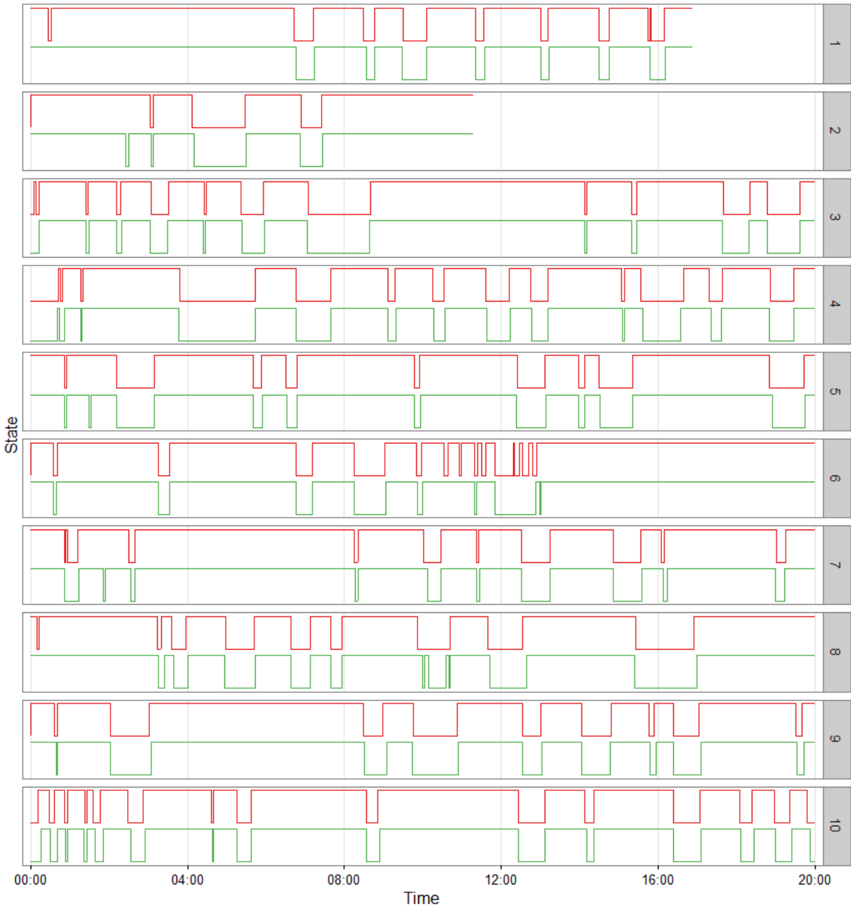
Fig. 61. Prius state estimation of validation trips. Red: Prediction, Green: Observed.
