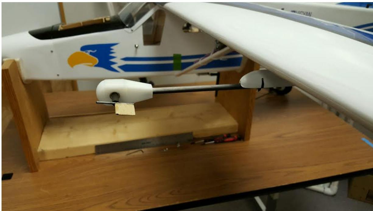
Figure 2.2 Forward Gust Sensor, a.k.a. The Bird
