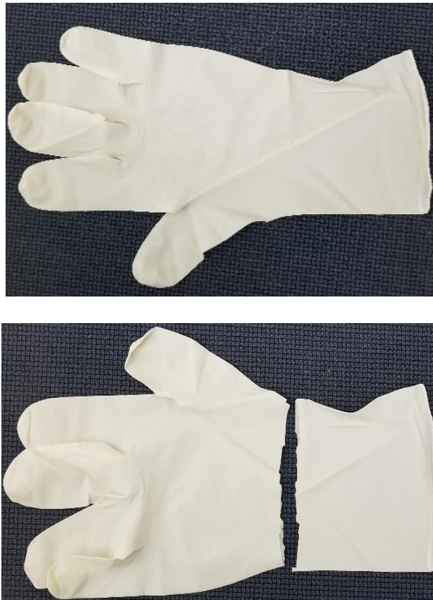
Fig. 19 Modified surgical glove used in the webbed three-fingered grasper of RoboCatch
