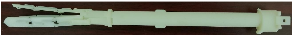
Fig. 29 Full assembly of the middle tube and the three-fingered grasper
