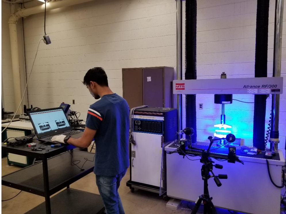
Fig. 4. 9 Digital Image Correlation Setup for Analysis of Four Point Bend test
