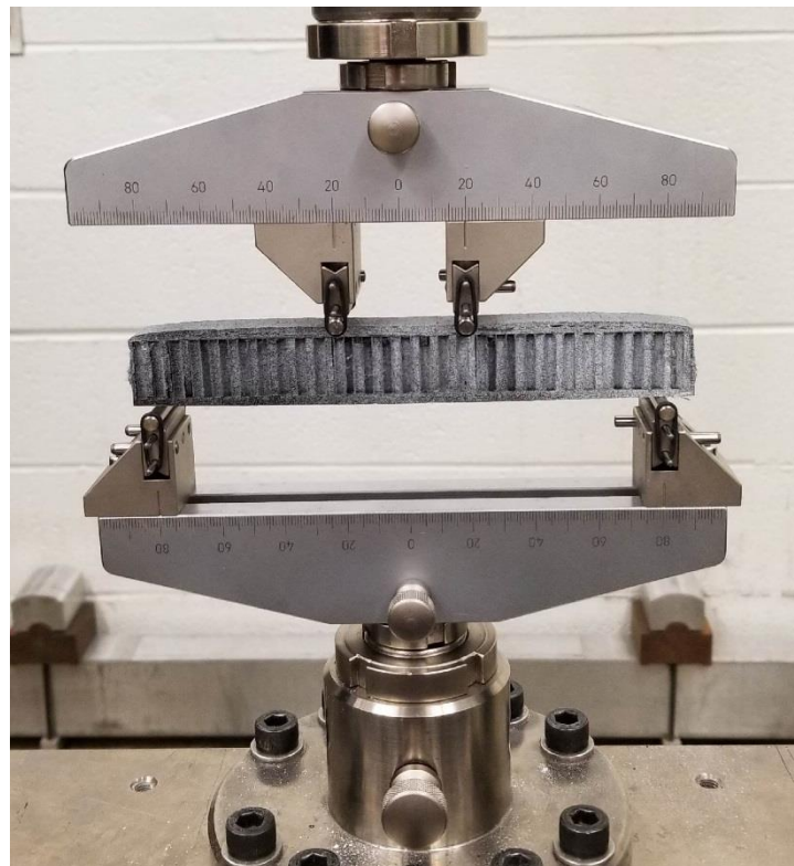
Fig. 4. 3 Test setup (four-point bend test)
