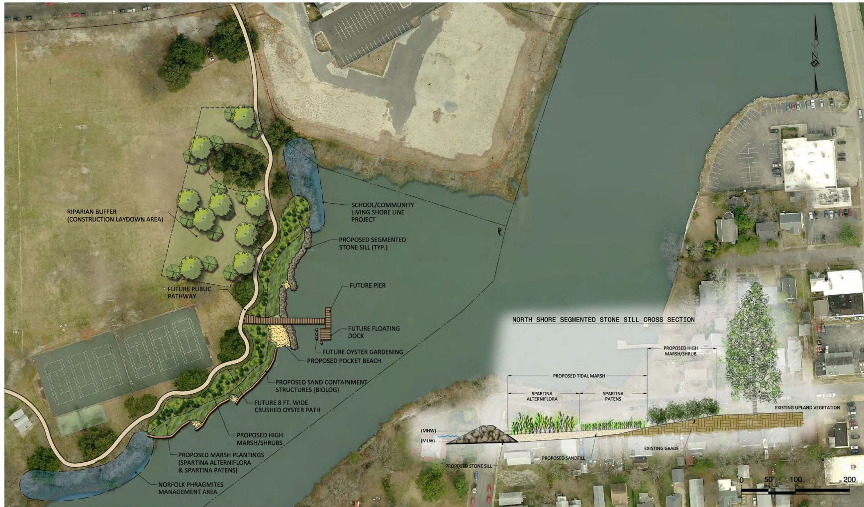
COLLEY BAY LIVING SHORELINE NORTH SHORE SEGMENTED STONE SILL & FRINGE MARSH WITH BIOLOGS
