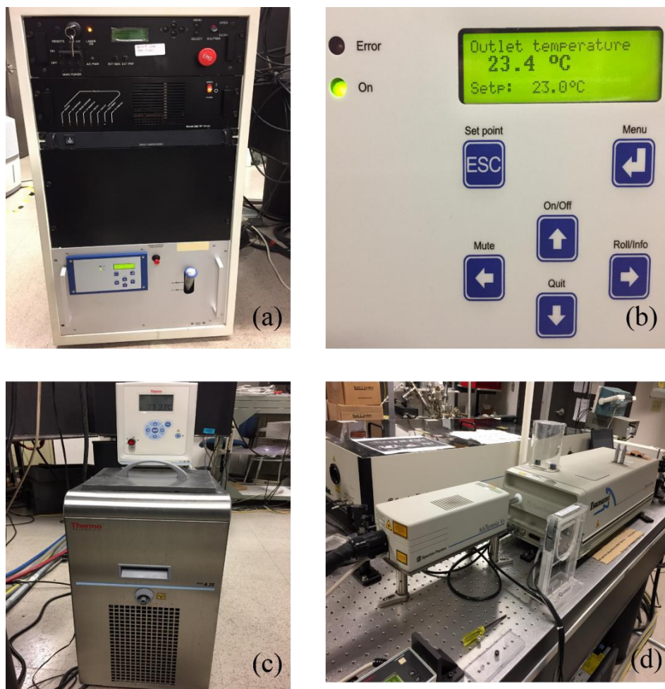
Fig. D.1. (a) power supply with chiller, (b) chiller temperature, (c) chiller for regen and oscillator and (d) pumping oscillator, oscillator, and regen.
