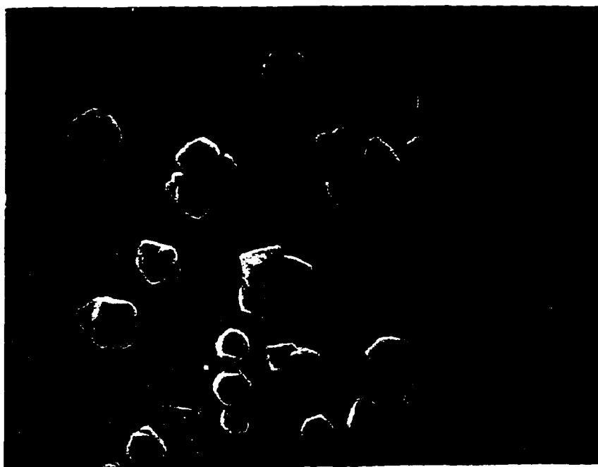
Figure 5.4 SEM picture of diamond particles grown by oxygen-acetylene flame technique
