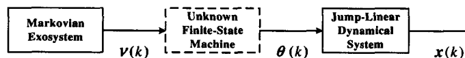
Figure 5.3: A jump-linear system driven by an unknown finite-state machine with a Markovian input.
