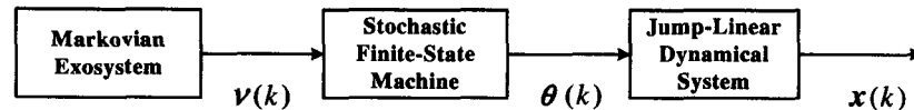
Figure 5.2: A jump-linear system driven by a stochastic finite-state machine with a Markovian input.
