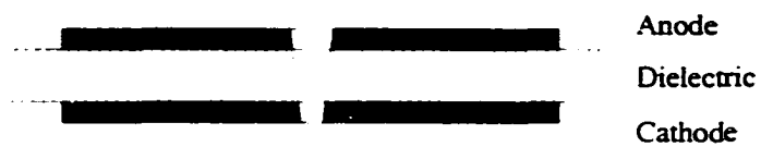
Figure (4.1) Typical MHCD sample
