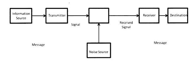
Figure 11. Shannon's (1948) General Concept of a Communication System
