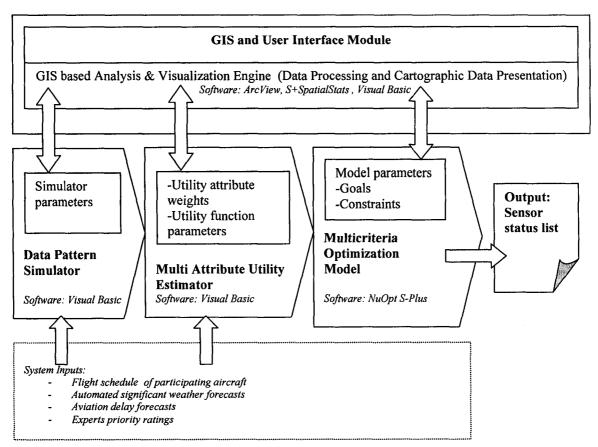
Figure 8 Components of TAMDAR DSS architecture
