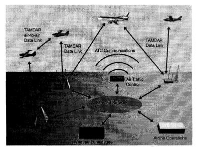
Figure 1 Architecture of the TAMDAR System.
