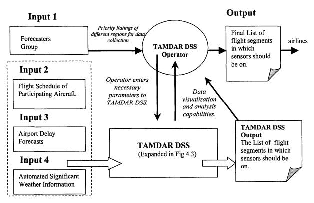
Figure 7 The TAMDAR DSS Architecture.
