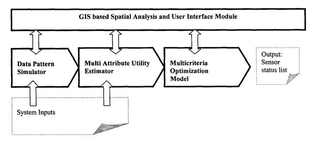
Figure 5 The TAMDAR DSS architecture
