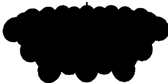
Figure 2.1 Schematics of the wall surface for optimized gas/wall interaction model for three-dimensional MD simulations. The line represents the center line of the model.
