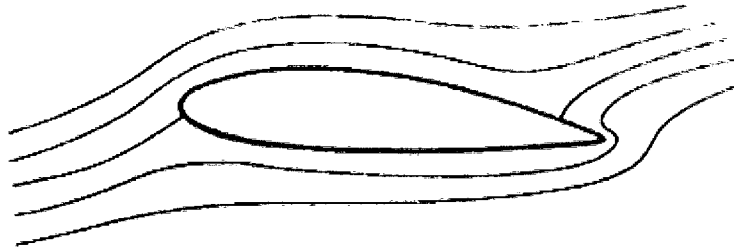
Figure 3.2: Streamlines of the Flow around an Airfoil with Zero Circulation, Stagnation Point on the Rear Upper Surface
