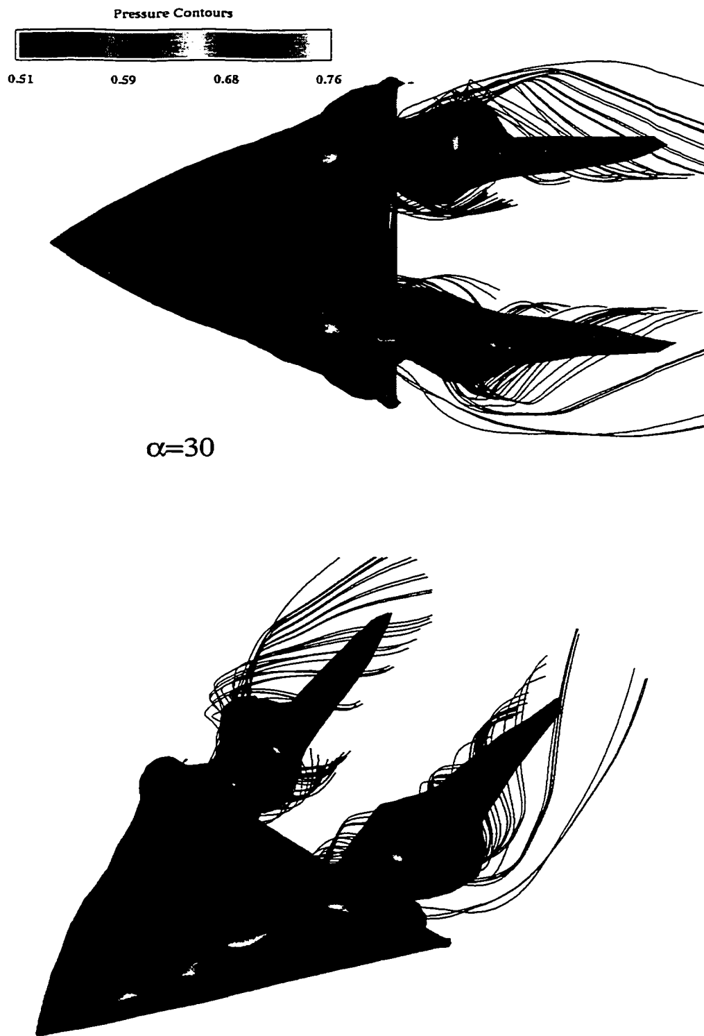
Figure 7.6: Particle traces and Mach number contours over the delta wing at \alpha = 30^\circ
