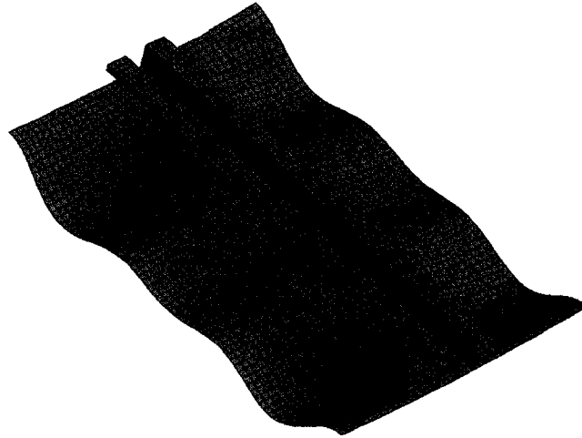
Figure 4. Local skin buckling mode for hat-stiffened panel
