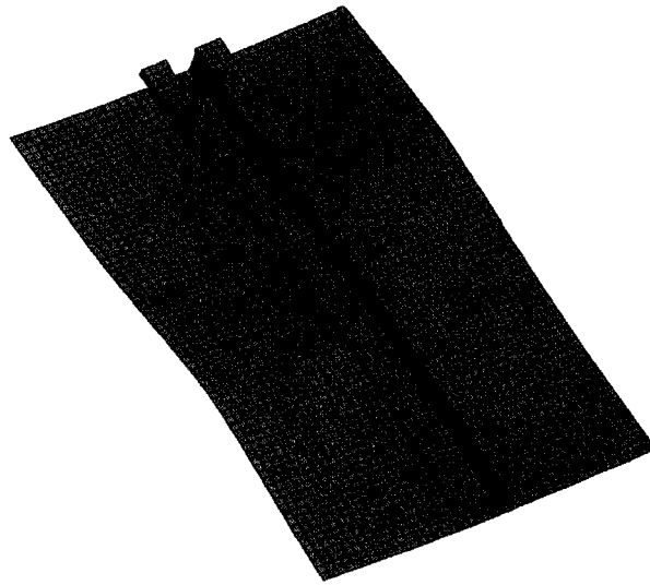
(a) Bonded stringer failure, P_f = 6,640 lbs
