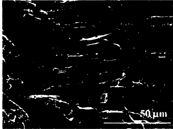
FIG. 14. Increased surface roughness due to higher laser fluence ( > 2.3 \text{ J/cm}^2 ) treatment.
