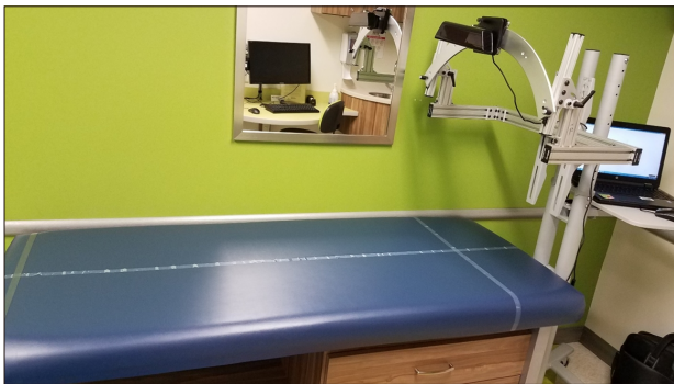
Fig. 1. ODU scanner, showing a laptop containing our proprietary software and markings on the exam table to allow consistent patient placement in the supine position.
