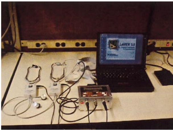
Fig. 1 VUR data acquisition system (VURDAS); the configuration shows two renal sensors, a wetness sensor and acquisition hardware.
