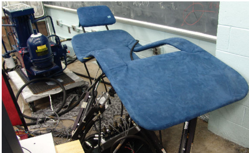
Figure 8: The 6-DOF Hydraulic Stewart Platform.
