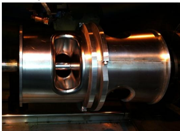
Figure 4: Cavity main body middle seam welding.
