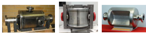
Figure 19: Proof-of-principle cavities: 4-rod cavity (left), double quarter wave cavity (middle), and rf-dipole cavity (right).
