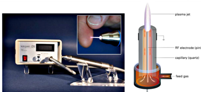
Fig. 35. Picture of INP kINPen 09 and a schematic diagram of the device (figure courtesy of INP Greifswald, Germany).
