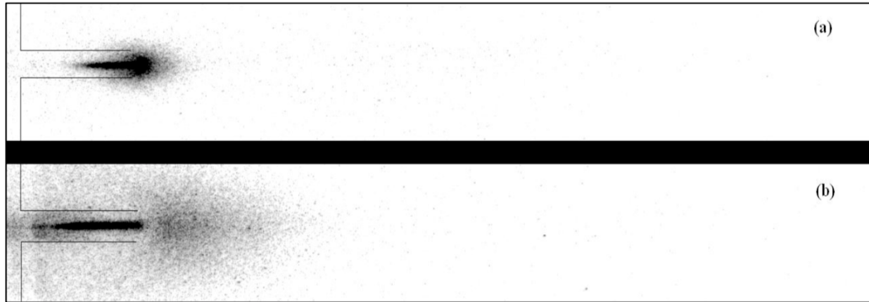
Figure 10. High-speed photographs of an FIW generated by introducing a discharge into a large-volume chamber at pressures a) 75 Torr and b) 25 Torr. The chamber is filled with helium. The applied voltage pulse was 7 kV, frequency: 5 kHz, and pulse width: 2 \mu s [46].
