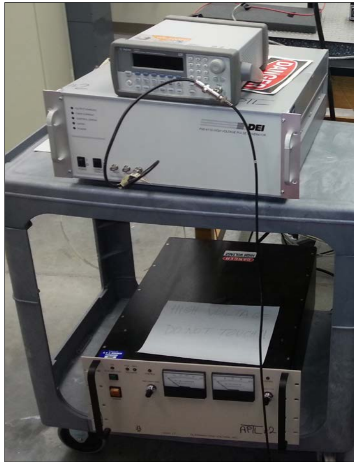
Figure 18. The photograph of the pulsed power supply consists of a high-voltage DC supply (bottom), high-voltage pulse generator (middle), and a 20MHz function/arbitrary waveform generator, Agilent 33220A (top).
