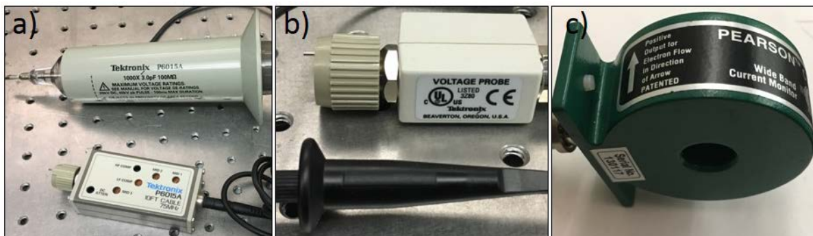
Figure 19. a) High-voltage probe, Tektronix P6015A, b) voltage probe, Tektronix P6139A, and c) Pearson current monitor 4100.
