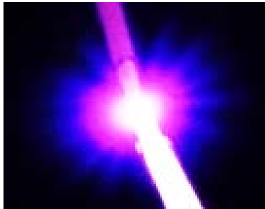
Figure 81. Image of plasma plume spreading over a Plexiglass surface with a thickness of 17 mm (Applied voltage: 7 kV, pulse width: 1000 ns, repetition rate: 7 kHz, He flow rate: 7 slm, Distance between the APPJ tube exit and the dielectric surface: 6 mm).
