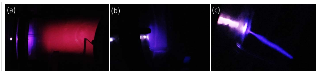
Figure 85. The transition of plasma from a diffuse glow discharge to corona discharge in a chamber filled with air at a) 200 mTorr with negative glow and positive column, b) at 1 Torr without the positive column, and c) at 3 Torr transitions to corona discharge (Applied voltage: 7 kV, pulse width: 1000 ns, repetition rate: 7 kHz, APPJ He flow rate: 7 slm, Distance between plasma jet exit tube and the chamber: 6 mm).
