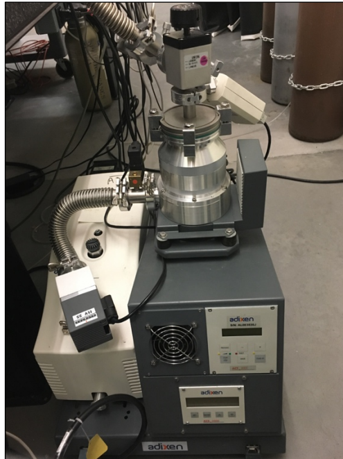
Figure 14. The photograph of the vacuum system Adixen ACP15 with Alcatel Adixen ACT200T control panel.
