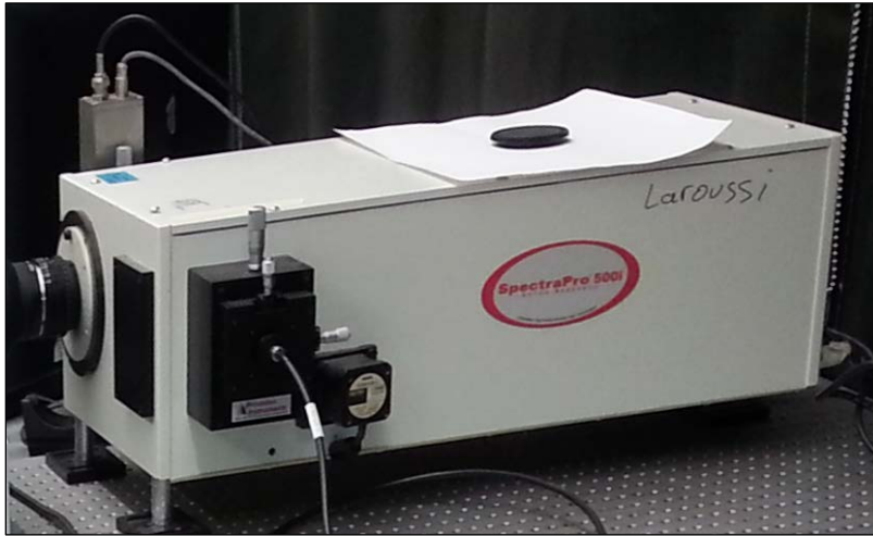
Figure 21. Spectrometer SpectraPro-500i with a PMT mounted on it with the capability of mounting ICCD as a complimentary photo-sensing device.
