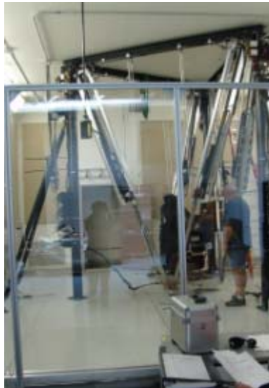
Figure 12: A 6-DOF Inverse Stewart Machine
