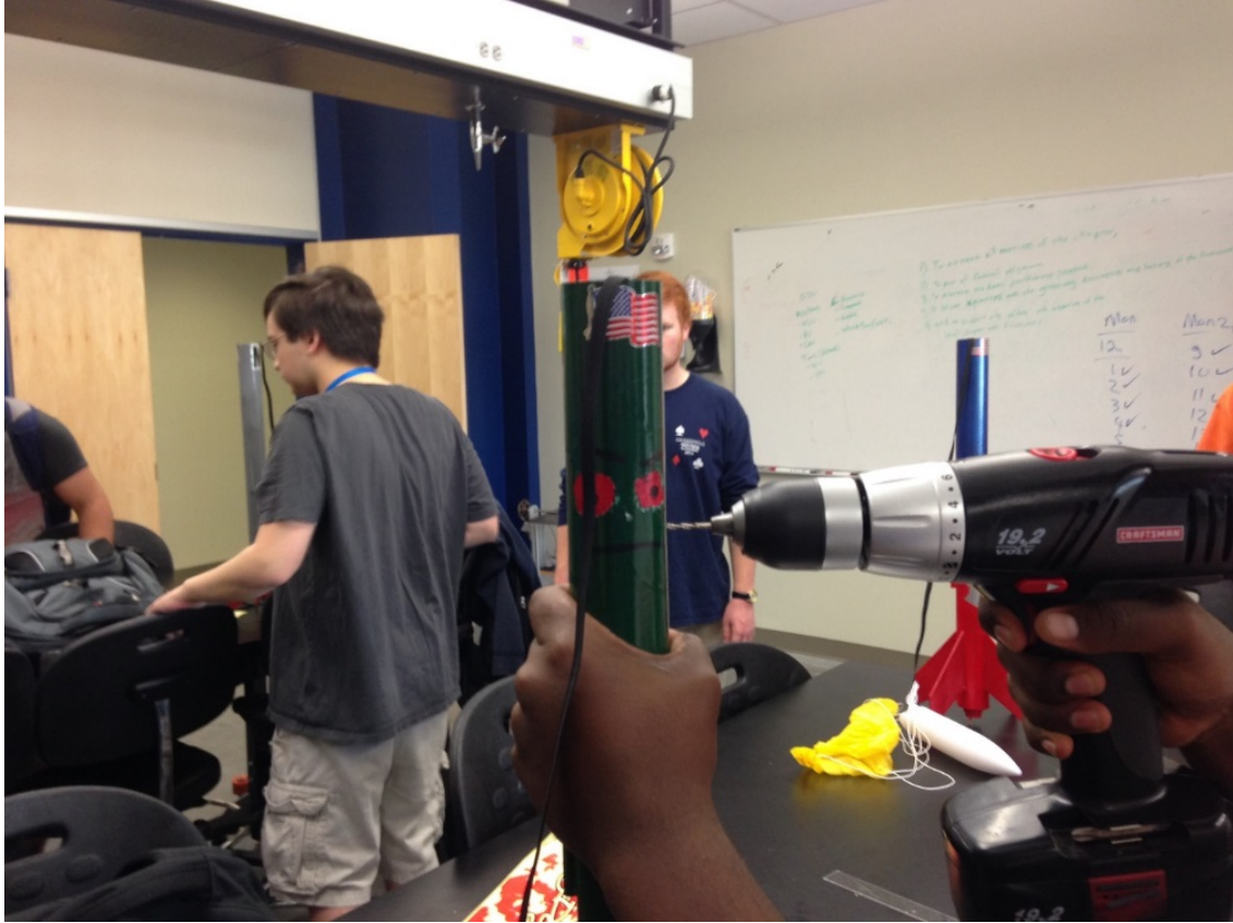
Figure 8B. Holes drilled to allow air for altimeter to work
