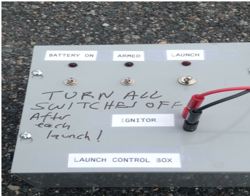
Figure 17. Home built launcher to reduce misfires and provide consistent current
