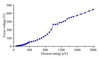
Figure 1: Focus voltage of the electron gun as a function of electron energy.
