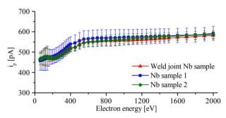
Figure 3: Primary electron beam current as a function of electron energy during SEY measurement of Nb sample and weld joint Nb sample. Statistical error bars are indicated.
