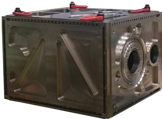
Figure 10: Prototype model of the helium tank.
