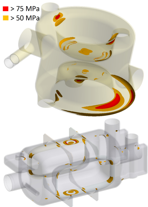
Figure 7: Stress on DQW (top) and RFD (bottom) cavities. The red locations require a further step in the assessment with the linearized stress.
