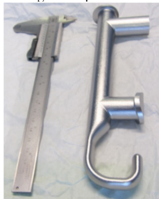
Figure 15: First prototype of the DQW HOM hook built at CERN.
