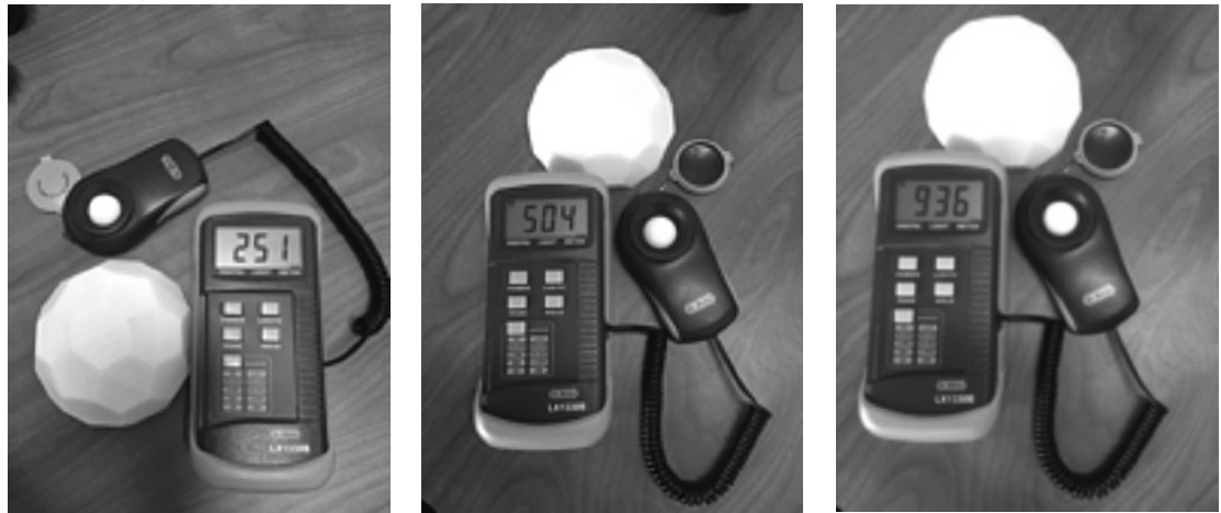
Figure 4: Photometer used to measure ambient light for the three treatments
