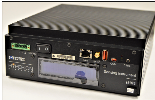
Figure 3.2: Micron Optics si-155 fiber optic interrogator.
