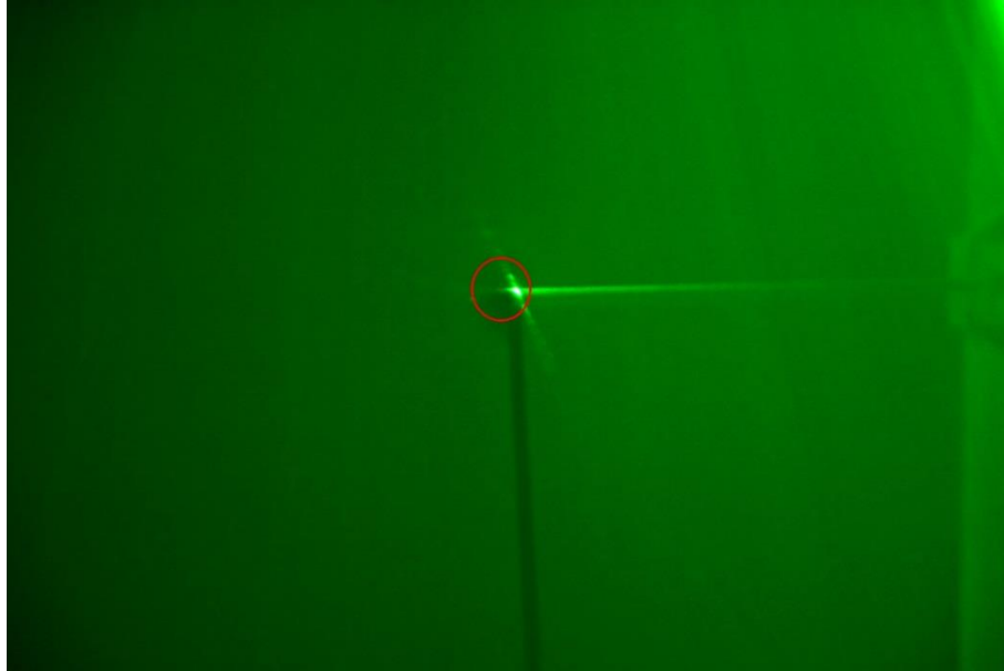
Figure 31 crosswise flow visualization during probe insertion 10.5 chord lengths downstream at a tunnel speed of 40m/s
