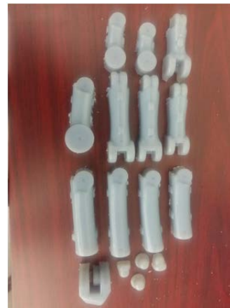
Fig. 4.12. (a) 3D Printed index finger, (b) Fingers covered in support material
