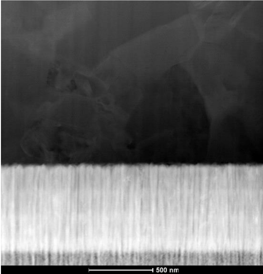
Figure 4.8 TEM image of CIGS solar cell sample
