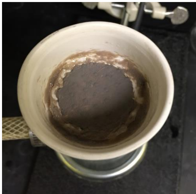
Figure 10: BNNT deposition in which edges of PCTE membrane curl under pressure
