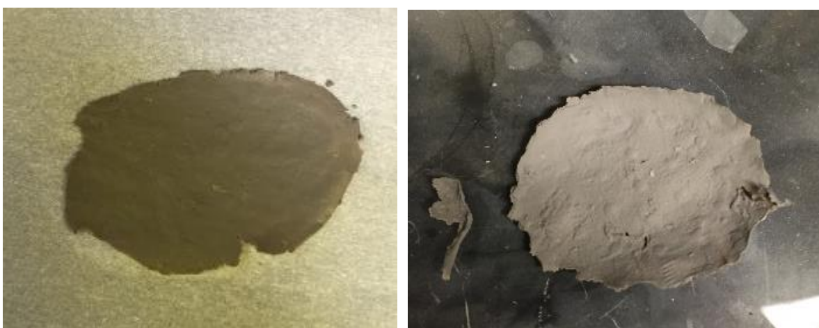
Figure 9: BNNT mat before drying on parchment paper (left) and after drying on hotplate (right)
