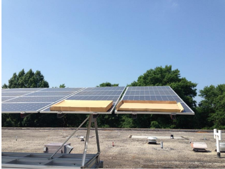
Figure 3.17: Shading arrangement for two shaded PV modules.
