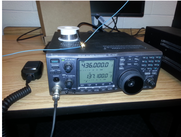
FIG. 2: Icom IC-910 conventional radio that is primarily used by Amateur Radio Operators for Satellite Communications.
