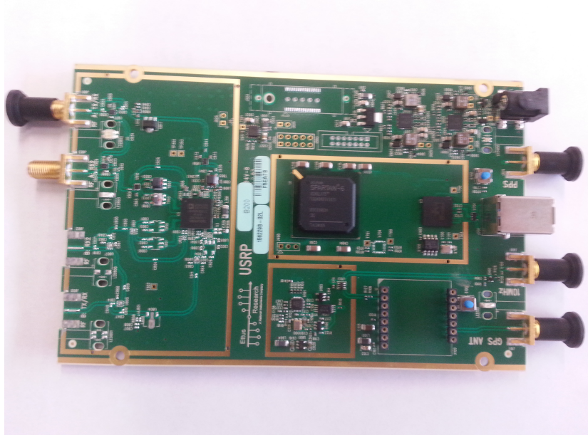
FIG. 4: USRP B200 software defined radio developed by Ettus Research.
