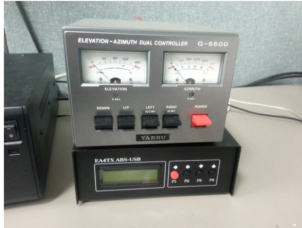
FIG. 7: Image of a Yaesu G-5500 rotator controller with a EA4TX computer interface. The G-5500 controls the motors on the rotator and the computer interface allows the computer to communicate with the controller.
