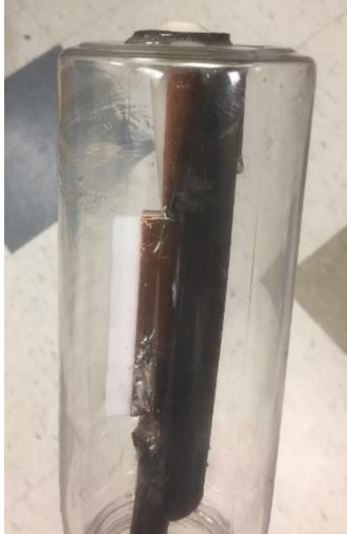
Figure 30: Antenna structure with a bottle housing
