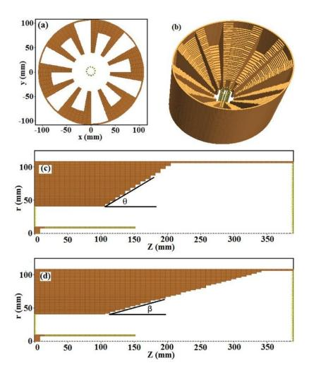
Figure 3-12. Rising-Sun magnetron with the anode block geometry chosen as the first configuration for quantitative performance evaluation with variable angle for short vanes (angle  $\beta$ ). (a) Cross sectional view in the r- $\varphi$  plane. (b) Three dimensional view for  $\beta$  equal to 15 degrees. (c) Cross sectional view of the long vanes in the r-z plane. (d) Cross sectional view of the short vanes in the r-z plane [47].
