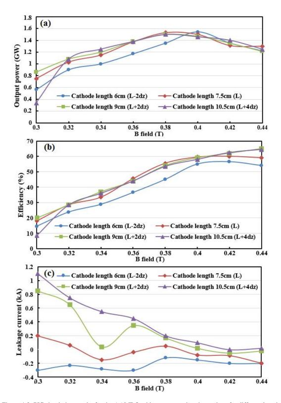
Figure 4-2. PIC simulation results for the A6 MDO with one comprehensive endcap for different length of cathodes. (a) The output power, as a function of the applied magnetic field, (b) Efficiency, as a function of the applied magnetic field, and (c) Leakage current, as a function of the applied magnetic field.
