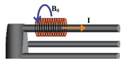
Figure 2-16. The axial current in the cathode strip and the corresponding azimuthal magnetic field lines [29].
