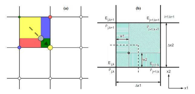
Figure 3-3. (a) Schematic of the scatter operation. (b) Graphical representation of the linear weighting on the 2-D structured Cartesian grid.
