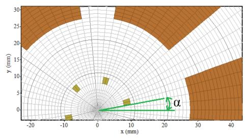
Figure 4-4. Angle between x-axis and first cathode (alpha).
