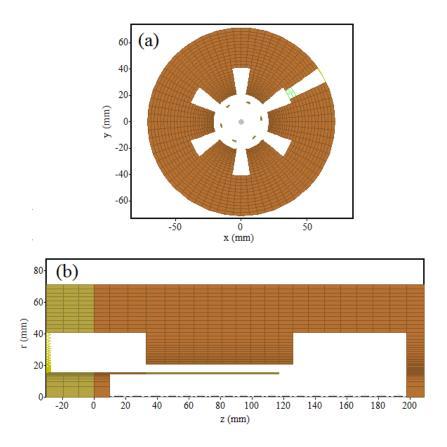
Figure 2-14. Geometry of A6 magnetron with transparent cathode. (a) r- $\theta$  plane cross section of A6 magnetron with transparent cathode. (b) r-z plane cross section of A6 magnetron with transparent cathode.
