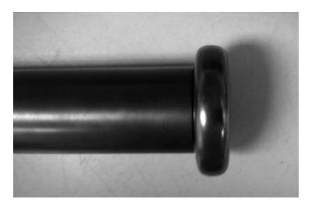
Figure 2-10. Photograph of endcap on solid cathode [5].
