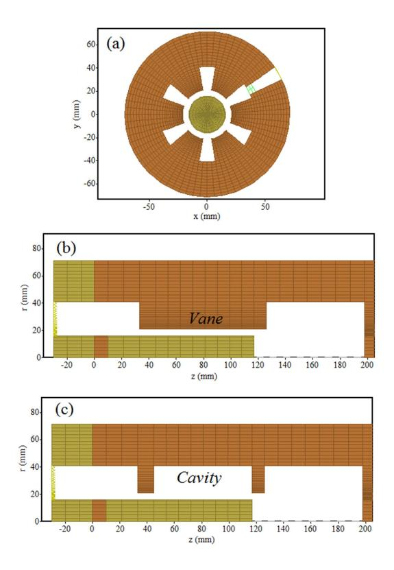
Figure 2-2. The different cross sectional view of A6 magnetron. (a) r- $\theta$  plane cross section. (b) r-z plane cross section at the  $\theta$  corresponding to center of vane. (c) r-z plane cross section at the  $\theta$  corresponding to center of cavity.
