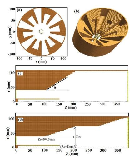
Figure 3-13. The second anode block geometry chosen for the Rising-Sun magnetron simulations with variable outer radius for short vanes  $(R_s)$ . (a) Cross sectional view in the r- $\varphi$  plane. (b) Three dimensional view for  $R_s$  equal to 75 mm. (c) Cross sectional view of the long vanes in the r-z plane. (d) Cross sectional view of the short vanes in the r-z plane [47].
