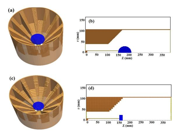
Figure 3-14. Geometry used for Rising-Sun MDO structures with different endcap geometries. (a) Three dimensional view with Bulb shape endcap, (b) Cross sectional view in the r-z plane with Bulb shape endcap, (c) Three dimensional view with cylindrical endcap, (b) Cross sectional view in the r-z plane with cylindrical endcap [47].
