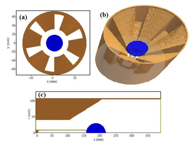
Figure 3-10. A6 MDO magnetron with bulb shape endcap. (a) Cross sectional view in the r- $\varphi$  plane. (b) Three dimensional view, (c) Cross sectional view in the r-z plane.
