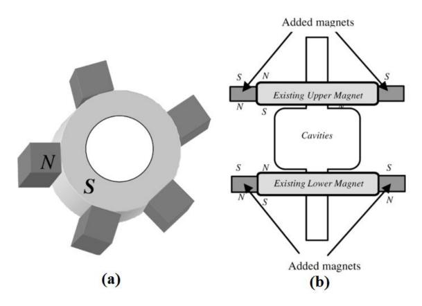
Figure 2-12. The arrangement of permanent magnets used for magnetic priming. (a) 3-D top view of the optimal magnetic priming in a Panasonic magnetron. (b) Side view of the typical axially symmetric, azimuthally varying magnetic field for a Toshiba magnetron [26].
