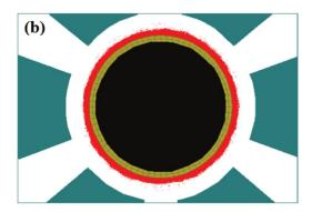
Figure 2-15. Electron prebunching in the transparent cathode. (b) Solid ring of electrons around the solid cathode [29].
