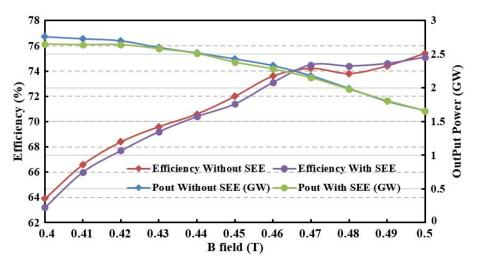
Fig 4-17. PIC simulation results for 12- cavity Rising-Sun magnetron with cylindrical end cap and cathode length 18 cm. The output power and device efficiency are shown as a function of the applied magnetic field with and without the inclusion of SEE.
