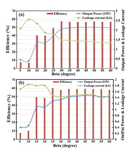
Figure 4-6. PIC simulation results for the 12-Cavity Rising-Sun Magnetron. The output power, device efficiency and leakage current are shown as a function of short vanes angle ( $\beta$ ). Applied magnetic fields of: (a) B = 0.42 T, and (b) B = 0.48 T were used [47].
