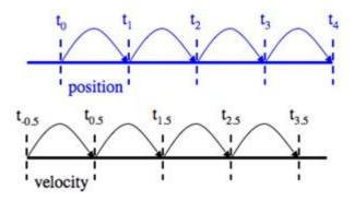
Figure 3-2. Schematic diagram of leap-frog method.
