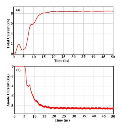
Figure 4-13. MAGIC-based simulation results for the 12-Cavity Rising-Sun Magnetron with a cylindrical endcap and 18cm cathodes (L+6dz) at a 0.45 T magnetic field. (a) Total current, and (b) Anode current [47].
