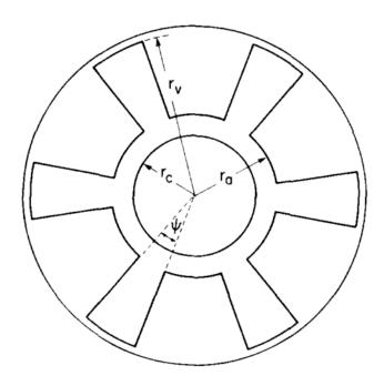
Figure 1-1. Basic configuration of a cylindrical magnetron [1].
