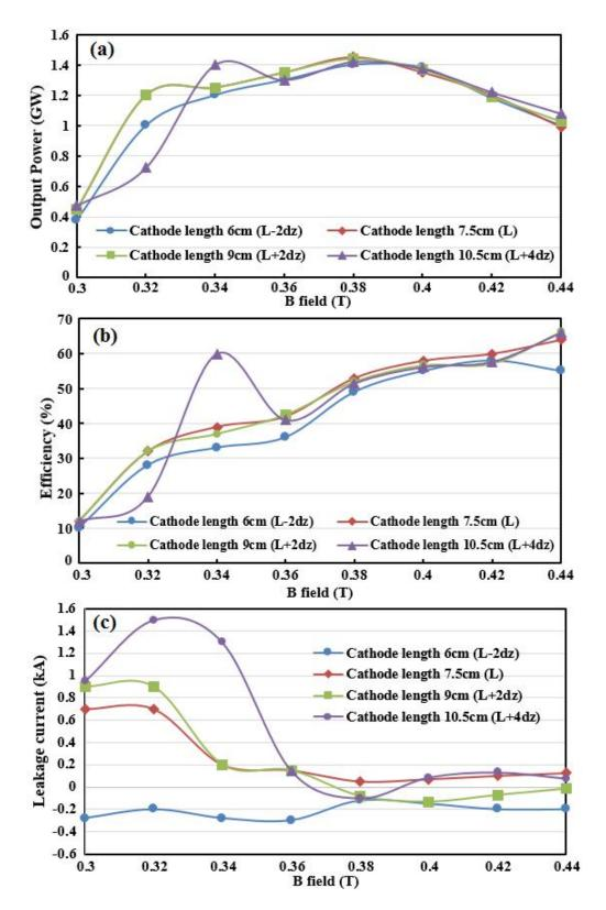
Figure 4-3. PIC simulation results for the A6 MDO with six individual endcaps for different length of cathodes. (a) The output power, as a function of the applied magnetic field, (b) Efficiency, as a function of the applied magnetic field, and (c) Leakage current, as a function of the applied magnetic field.
