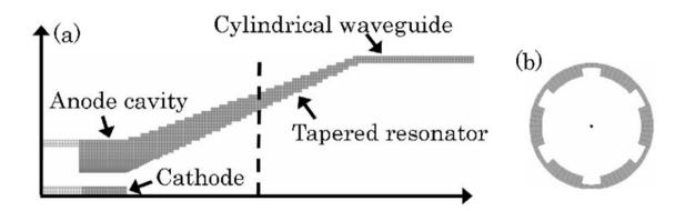
Figure 2-4. Geometry of early Russian MDO. (a) The z-r cross section, (b) the r- $\varphi$  cross section obtained at the dashed-line position [4].
