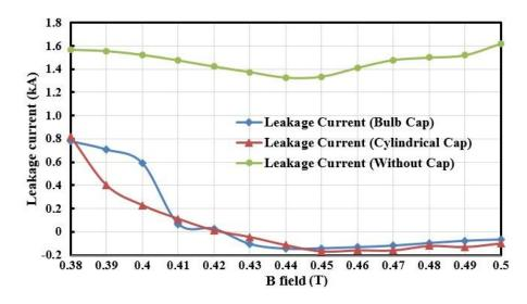
Figure 4-9. Leakage current of 12-Cavity Rising-Sun Magnetron for three different cathode structures. These structures were without any endcap, with a bulb-shaped cap, and with a cylindrical endcap [47].
