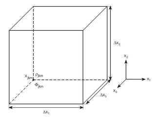
Figure 3-6. Computational mesh for electrostatic mesh [6].
