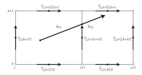
Figure 3-5. Current deposition for a multi-cell particle motion [6].
