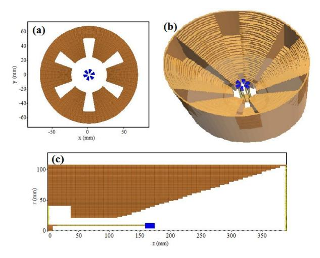
Figure 3-11. A6 MDO magnetron with six individual endcaps. (a) Cross sectional view in the r- $\varphi$  plane. (b) Three dimensional view, (c) Cross sectional view in the r-z plane.
