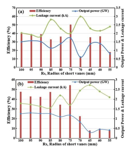
Figure 4-7. PIC simulation results for the 12-Cavity Rising-Sun magnetron. The output power, device efficiency and leakage current are shown as a function of the parameter  $R_s$ . As with figure 3-13, applied magnetic fields of: (a) B = 0.42 T, and (b) B = 0.48 T were used [47].
