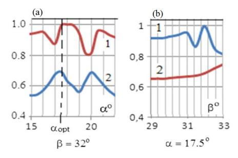
Figure 2-8. Dependence of radiation power P/Pmax (1) and efficiency (2) of UNM MDO on vanes angles. (a) angle  $\alpha$  (b) angle  $\beta$  [3].
