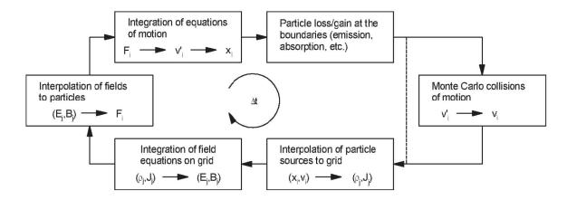
Figure 3-1. Particle-In-Cell computational cycle [6].
