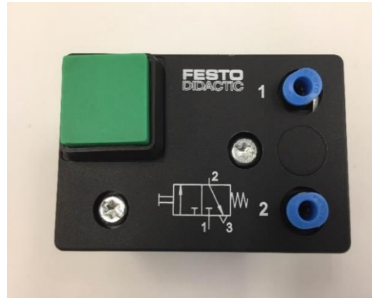
Fig. 6. Air Switch in Pneumatic Lab.
