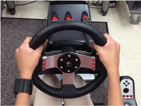
Position of the vibrotactile belt on the posterior side of the hand.
