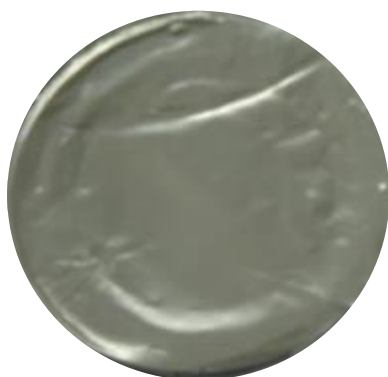
Proton-sensing film placed at anode facing the solution in the center Teflon chamber ( N' ) site.
