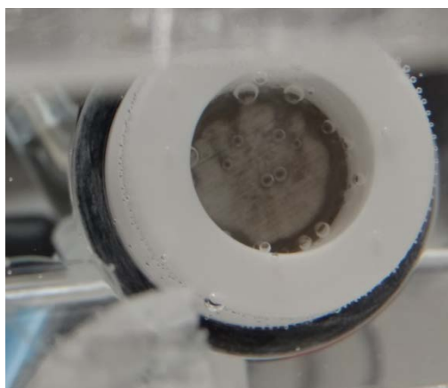
Figure 11. Teflon center chamber (with Al-Tf-Al membrane) after 10 hours electrolysis. Formation of gas bubbles and significant proton activity was noticed on the aluminum film surface at the P_1 site.
