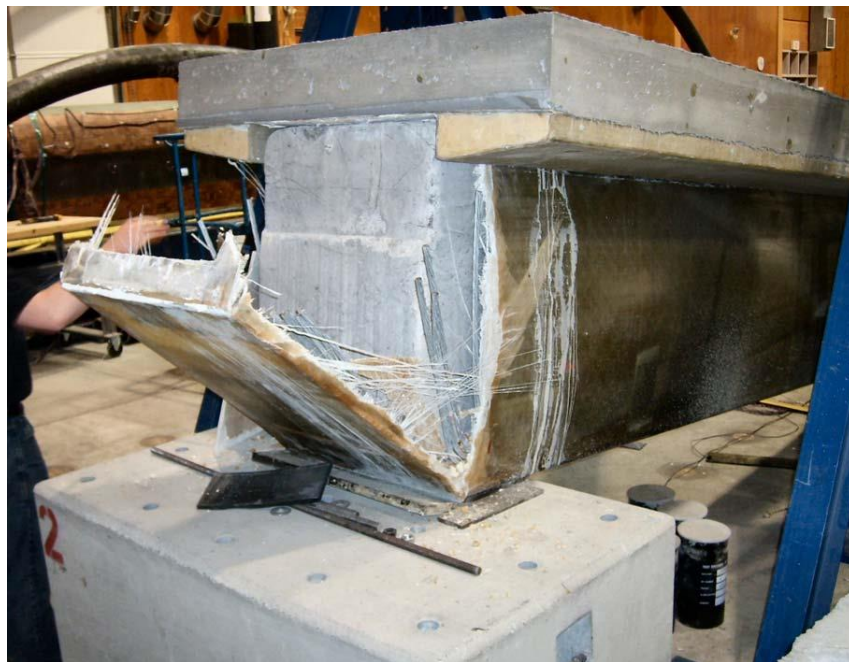
Figure 24. Premature failure of HCB due to detachment of tension reinforcement [10]
