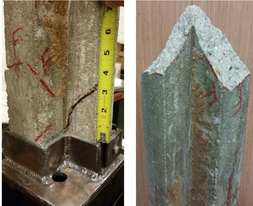
Figure 68. Final crack pattern for SM04
