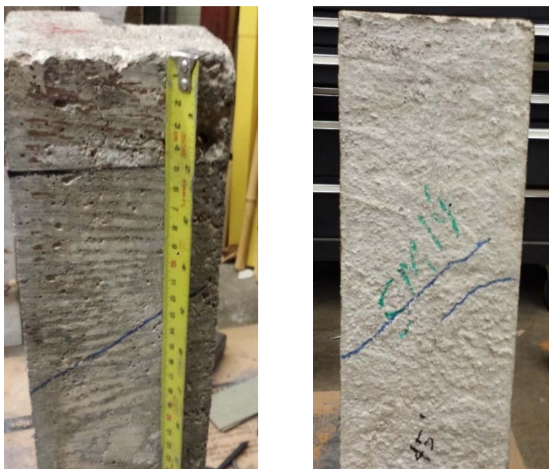
Figure 91. Final crack pattern of SM14
