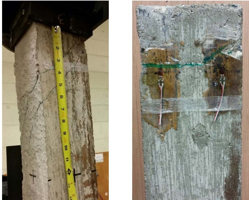
Figure 66. Final rack pattern for SS03
