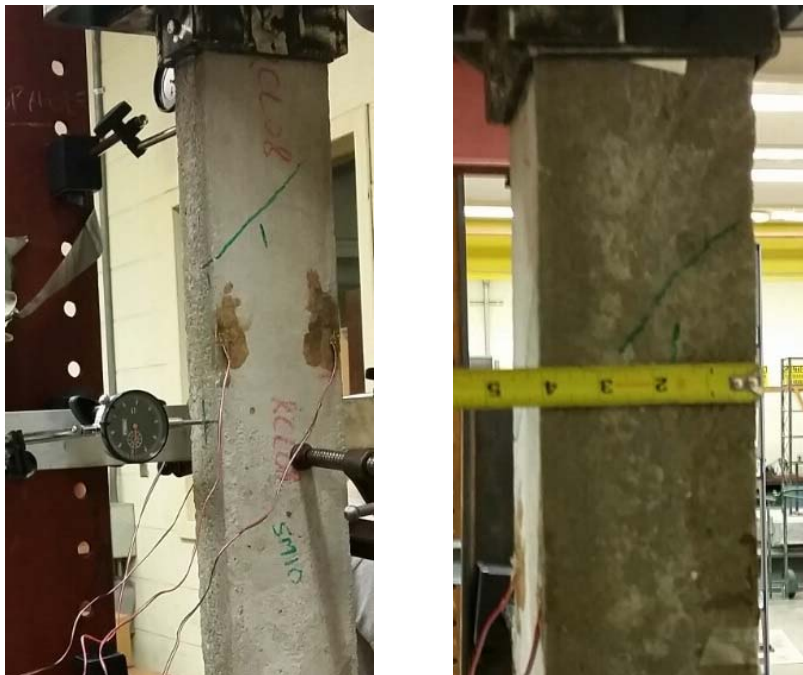
Figure 81. Final crack pattern of SM10
