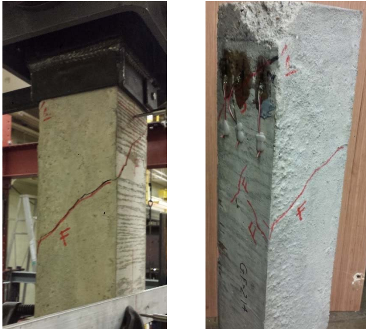
Figure 63. Final crack pattern of SS02
