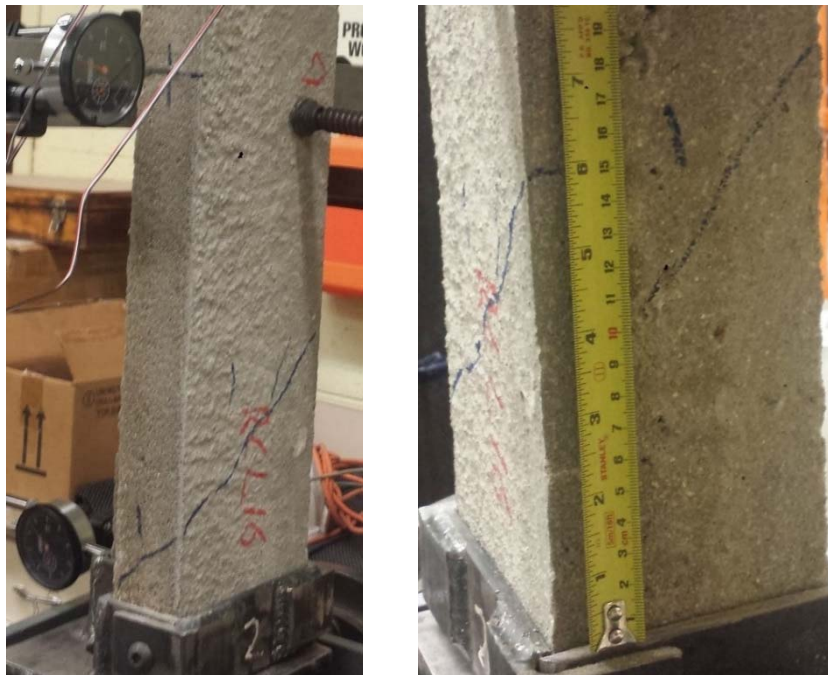
Figure 104. Final crack pattern of SM19
