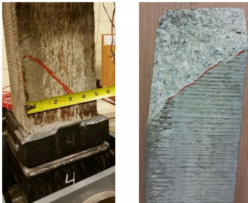
Figure 60. Final crack pattern of SS01
