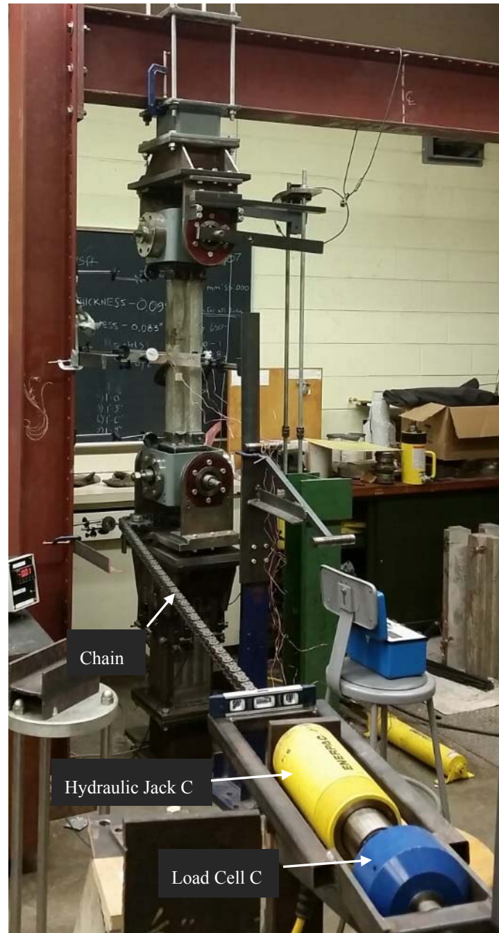
Figure 48. Torsion test setup for spandrel members
