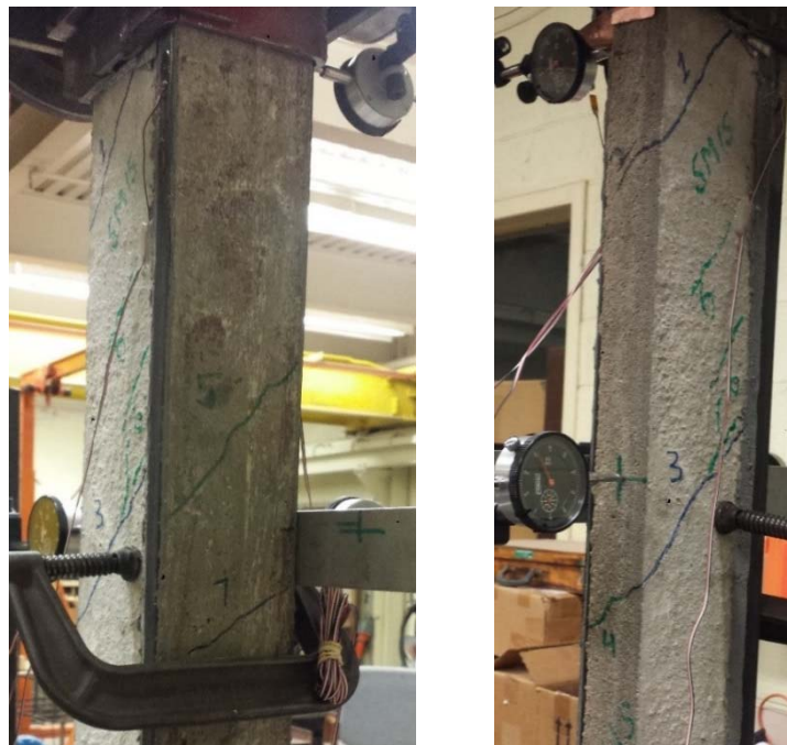
Figure 94. Final crack pattern of SM15
