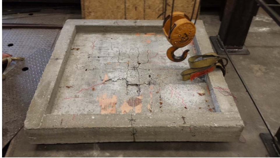
Figure 109. Bottom view of SL01 after test
