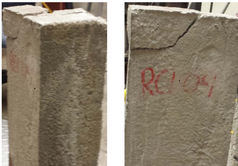
Figure 78. Final crack pattern of SM09
