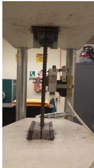
Figure 7. Typical rebar test setup
