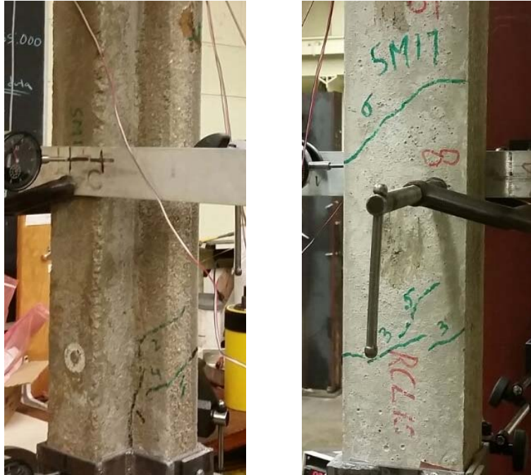
Figure 99. Final crack pattern of SM17
