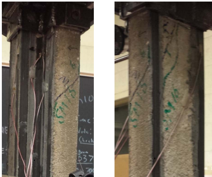
Figure 97. Final crack pattern of SM16
