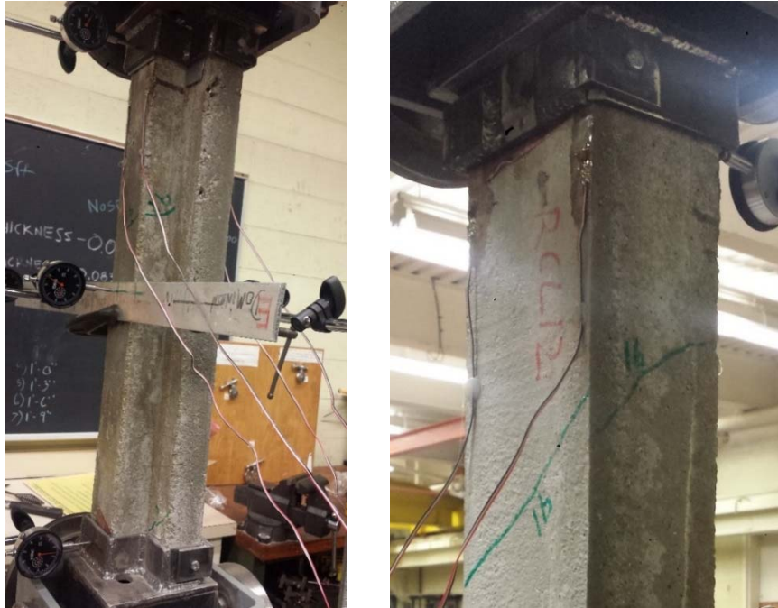
Figure 86. Final crack pattern of SM12
