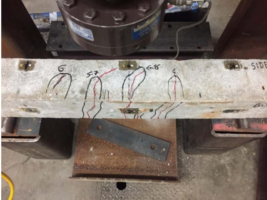
Figure 40. Cracking pattern of Beam 1
