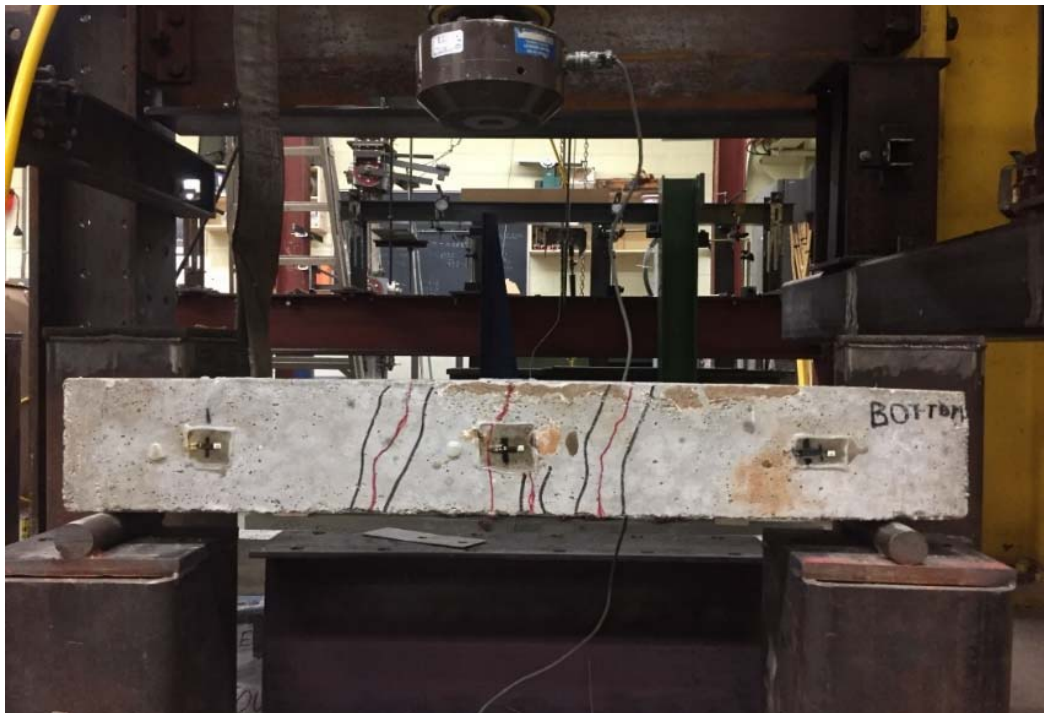
Figure 41. Cracking pattern in bottom surface of beam 1 after testing.
