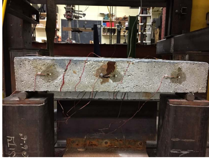
Figure 48. Cracking pattern in bottom surface of Beam 2 after test
