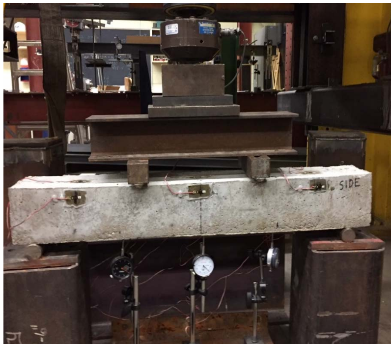
Figure 38. Test Setup for Two-point Load system
