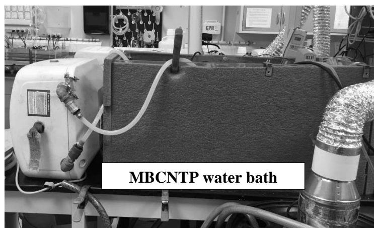
Figure 3 14 - MBCNTP water bath after insulation.
