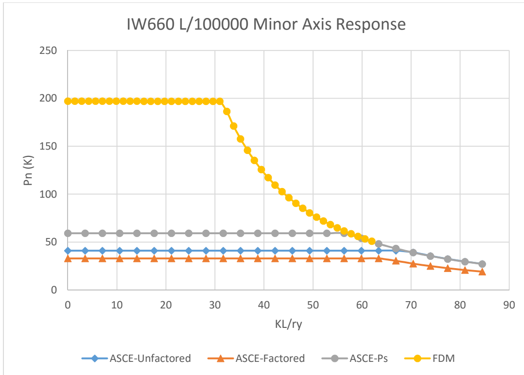
Fig. 71 Load vs. slenderness ratio for minor axis for ASCE LRFD Pre-Standard vs. FDM. L/100000
